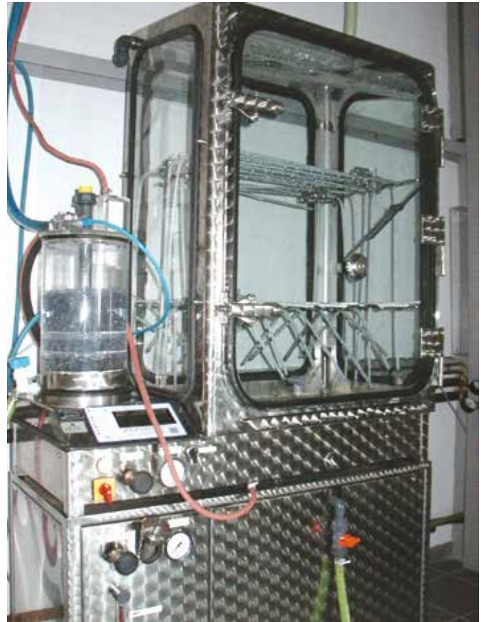
Environmental ageing chamber for ammonia atmosphere ageing
