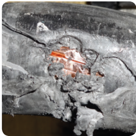
Major cable damage caused by thread contact
